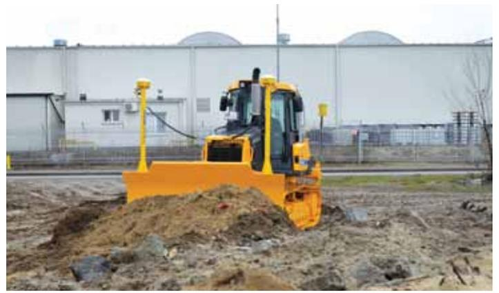
The dual path Hydrostatic Drive System allows for variable speed and steer control without the need to shift gears.
