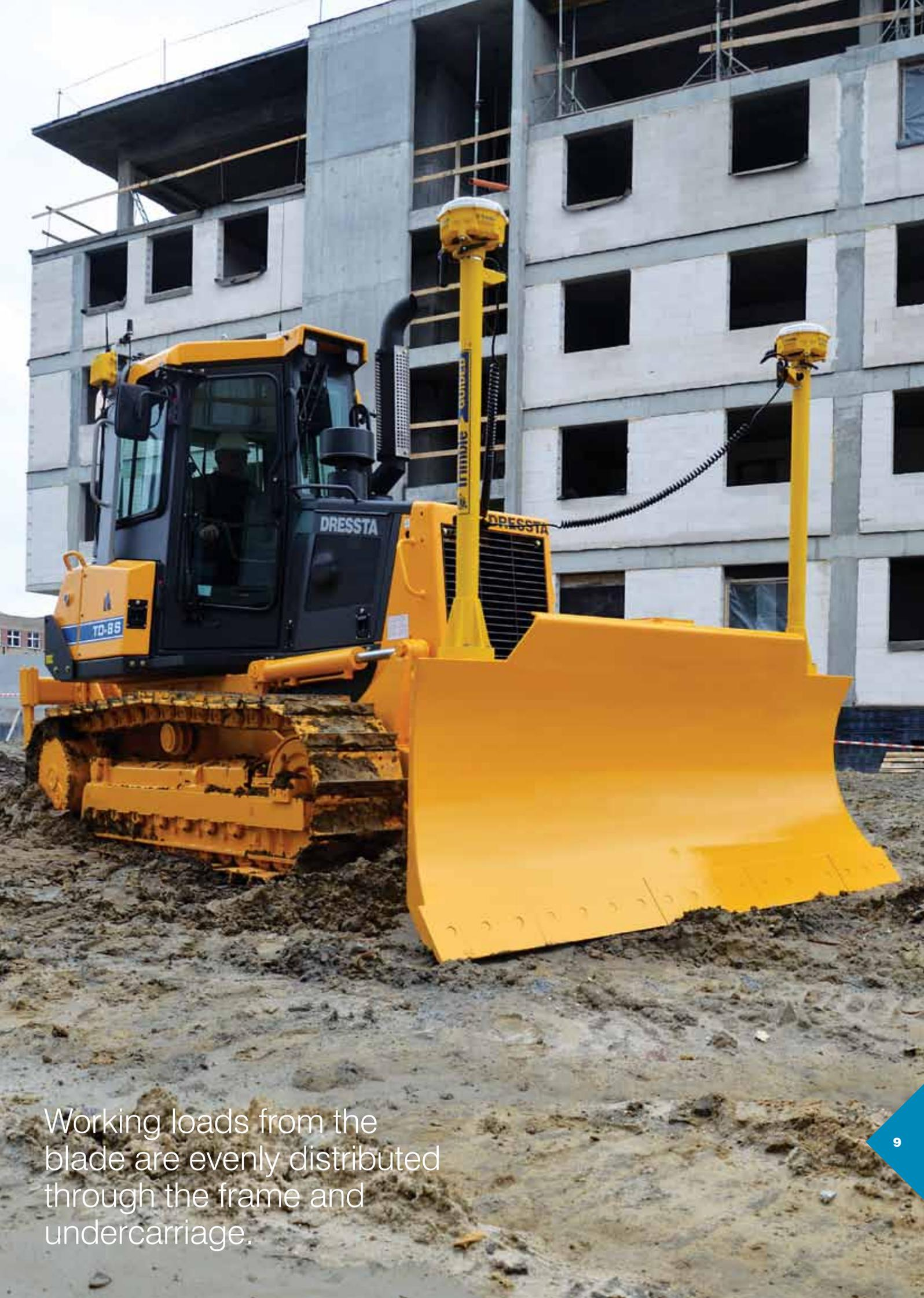
Working loads from the blade are evenly distributed through the frame and undercarriage.
