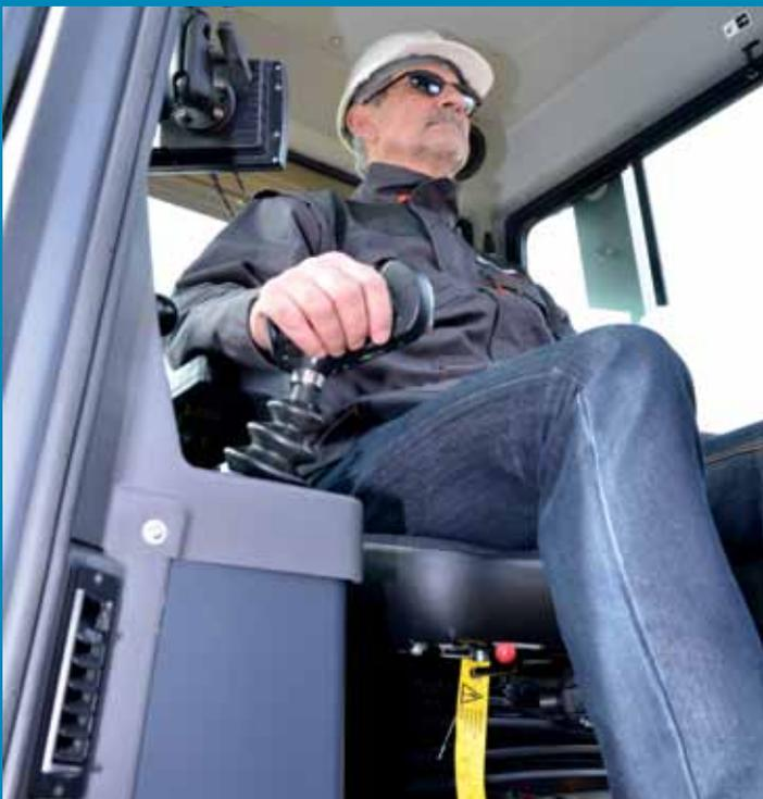
The all new hexagonal cab provides 30% more space and features full sound suppression. The cab is FOPS certified while the machine incorporates an additional two post ROPS protection system. Cab features include:
